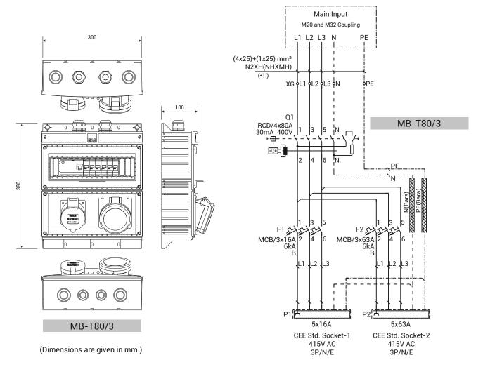
■In case of using 63A CEE Norm socket, "pilot contact" interlocking circuit should be applied. For details, please refer to page 60.
