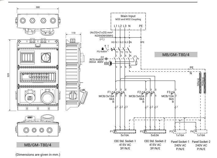
■In case of using 63A CEE Norm socket, "pilot contact" interlocking circuit should be applied. For details, please refer to page 60.
