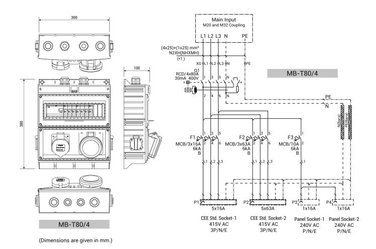
■In case of using 63A CEE Norm socket, "pilot contact" interlocking circuit should be applied. For details, please refer to page 60.
