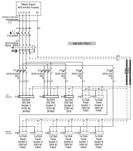
■Supply cable is for recommendation purposes and not within the scope. Cable type and cross-section should be determined by taking into consideration the voltage drop, temperature and short circuit calculations.
